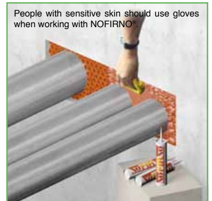
15) A cloth is sprayed with water. Note: do not use soap water! The cloth is used to press down the sealant layer. Pressing down the NOFIRNO® sealant in a stiff way is absolutely vital for the mechanical stability of the sealing system.
