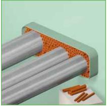
8) Single filler sleeves are used to fill the remaining small spaces in the set of fillers. Filling these spaces is of utmost importance to obtain a very tight fit of the filling inside the conduit frame.
