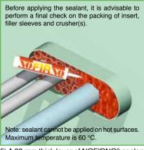
5) A 20 mm thick layer of NOFIRNO® sealant is applied at each side of the conduit. Clean and dry the conduit opening and the pipes thoroughly, and remove any dirt, rust or oil residues before applying the sealant.
