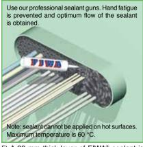
5) A 20 mm thick layer of FIWA® sealant is applied at each side of the conduit. Clean and dry the conduit opening and the cables thoroughly, and remove any dirt, rust or oil residues before applying the sealant.
