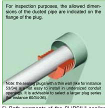
5) Both segments of the SLIPSIL® sealing plug are placed around the ducted pipe and then pushed into the conduit sleeve as far as the first serration. The first serration is smaller than the other serrations to make this procedure very easy.
