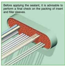
4) Push the insert/filler sleeves into the conduit in such a way as to leave about 20 mm free space at the front. The whole set of insert and filler sleeves should fit tightly into the conduit to provide sufficient mechanical stability.
