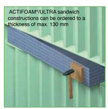
2) To fit the system to the height of the gap sheets of ACTIFOAM® with same are varying thickness (10,15, 20, 25 mm) are used. Top/bottom always with a cover of RISE®/ULTRA. The sandwich can be hammered in with the aid of a piece of wood.
