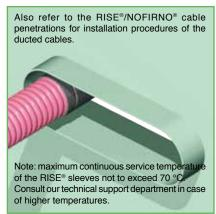
1) The cables can be ducted through the conduit sleeve/frame in random order.
