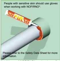
2b) A layer of NOFIRNO® sealant is applied at each side of the conduit. Clean and dry the inside of the conduit sleeve and the outside of the plastic pipe thoroughly, removing any dirt, rust or oil/lubricant residues before applying the sealant.
