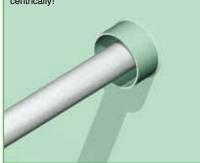
1) Before starting the installation procedure, any dirt, oil residues or welding spots should be removed from the conduit sleeve. For ease of installation, it is advisable to grind out the front side of the sleeve. Ask for the fitting CSD® conduit sleeves.
