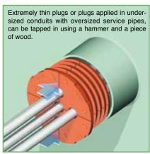
7) Then the four segments of the SLIPSIL® multi-sealing plug are pushed by hand evenly, serration by serration, further into the conduit sleeve.
