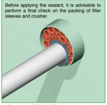
4) Push the NOFIRNO® filler sleeves into the conduit in such a way as to leave about 20 mm free space at the front. The whole set of filler sleeves should fit tightly into the conduit to provide sufficient mechanical stability.
