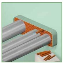
9) The single filler sleeves are inserted in the open spaces. At this stage they can generally be pushed in by hand. At the final stage to create a very tight fit of the whole set of fillers, the sleeves can be inserted with the help of a flat nose pliers.
