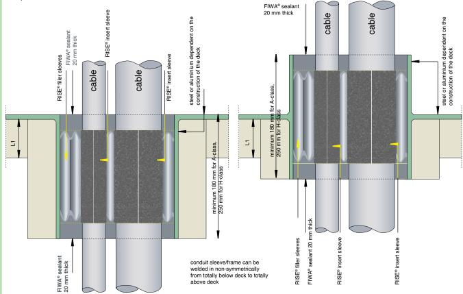
The FIWA® sealant may be substituted with NOFIRNO® sealant.
