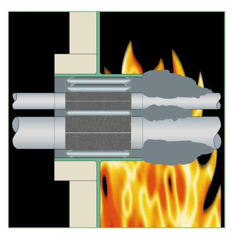
RISE® multi-cable penetrations are the best alternative for the casting compounds and block systems used in fire-rated/watertight bulkheads and decks. RISE® multi-cable penetrations offer a most simple way of installation.
