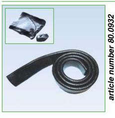
CONDUCTON® flexible rubber has been developed for the RISE®/EMC multi-cable transits and is used to fill the cavity around the ducted cables in the conduit sleeve, instead of making use of the putty. This rubber can be molded by hand and offers the highest attenuation.
