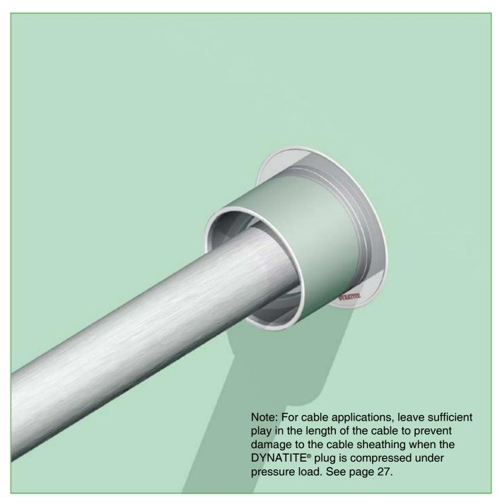
1) During welding, care has to be taken that no welding spots will get on the coated inner surface of the conduit sleeve. This would have an impact on the functionality of the system. Once the DYNATITE® conduit sleeve is welded into the partition, the pipe/cable can be passed through. The pipe/cable has to be ducted straight and centrically. This is of utmost importance for the displacement of the rubber when the pressure load occurs.
