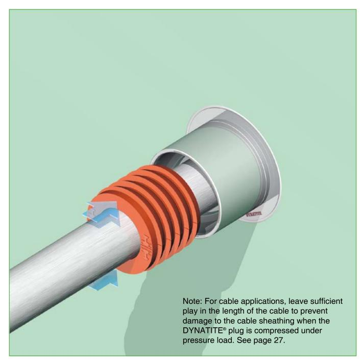
5) Both segments of the DYNATITE® sealing plug are placed around the ducted pipe/cable, then pushed into the conduit sleeve as far as the first serration. The first serration is smaller than the other serrations to make this procedure very easy. Both halves are then pushed by hand evenly, further into the DYNATITE® conduit sleeve. The inlet of the DYNATITE® conduit sleeve is rounded off to avoid any damages to the plug during insertion.
