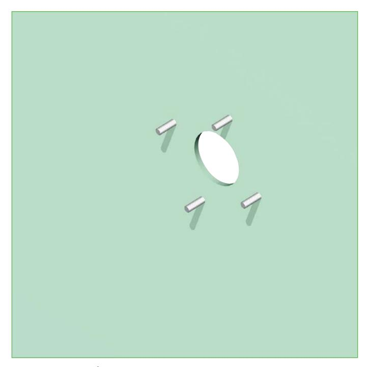
1) When DYNATITE® conduit sleeves for bolting are going to be used, a hole has to be cut in the partition to the size of the opening in the retainer flange of the DYNATITE® conduit sleeve. Threaded ends have to be welded to the partition in accordance with
