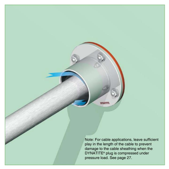
4) Once the DYNATITE® conduit sleeve is fixed against the partition, the pipe/cable can be passed through. The pipe/cable has to be ducted straight and centrically. This is of utmost importance for the displacement of the rubber when the pressure load occurs. Before starting the installation procedure, any dirt or oil residues should be removed from the conduit sleeve. The inside wall of the conduit sleeve is treated with CSD® lubricant to make installation of the DYNATITE® plug most easy.
