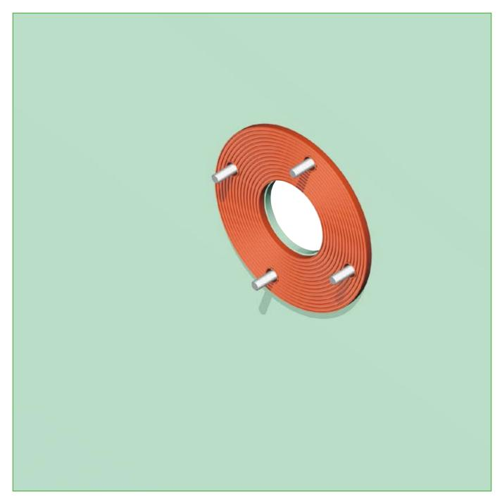
2) A fitting NOFIRNO® gasket is placed over the threaded ends against the partition.
