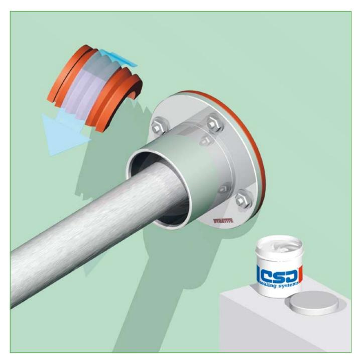
6) The segments of the DYNATITE® sealing plug are also treated with CSD® lubricant on the outside.
