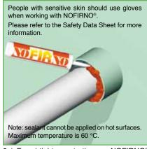
2a) For airtight penetrations, a NOFIRNO® sealant layer with thickness min. 5 mm is applied at both sides of the penetration. For watertight penetrations the sealant layer has to be 20 mm thick at both sides of the penetration.
