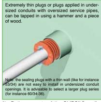
6) Both segments of the SLIPSIL® sealing plug are placed around the ducted pipe and then pushed by hand evenly, serration by serration, into the conduit sleeve.
