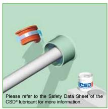
4) The RISE®/ULTRA C-FIT crusher should be inserted into the conduit sleeve over a length which corresponds with the length of the SLIPSIL® sealing plug. The segments of the SLIPSIL® sealing plug are treated with CSD® lubricant on the outside.
