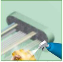
7) To smooth the surface of the FIWA® sealant layer, a cloth is sprayed with water. This prevents the sealant from sticking to the cloth. Note: do not use soap water!
