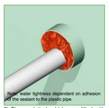
7) The conduit should be overfilled with NOFIRNO® sealant, because some sealant will be pushed between and into the empty filler sleeves during further finishing. This will contribute to obtain higher tightness ratings.
