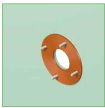
2) A fitting NOFIRNO® gasket is placed over the threaded ends against the partition. The DYNATITE® conduit sleeve can then be positioned. Avoid excessive forces on tightening of the NOFIRNO® gasket to guarantee tightness on long term.
