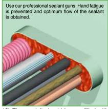
13) The conduit should be overfilled with NOFIRNO® sealant, because some sealant will be pushed between and into the empty filler sleeves during further finishing. This will contribute to obtain higher tightness ratings.
