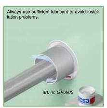
2) The inside wall of the conduit sleeve is treated with CSD® lubricant over its full length. The inlet of the DYNATITE® conduit sleeve is rounded off to avoid any damages to the plug during insertion.
