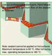
5) A 20 mm thick layer of NOFIRNO® sealant is applied at each side of the conduit. Clean and dry the conduit opening, and remove any dirt, rust or oil residues before applying the sealant.
