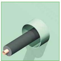
1) For fire rated penetrations of pre-insulated pipes (for instance for chilled water lines), by applying RISE®/ULTRA there is now no need to remove the insulation inside the penetration. This prevents condensation problems.
