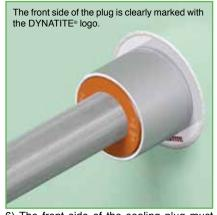
6) The front side of the sealing plug must be flush against the front side of the conduit sleeve. This proves that the back side of the plug is positioned against the retainer ring inside the conduit sleeve.
