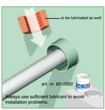
3) The inside surfaces of both segments of the DYNATITE® sealing plug are then treated with CSD® lubricant.
