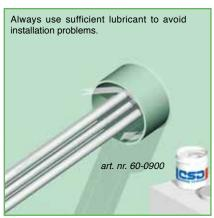
2) Then the inside wall of the conduit sleeve is treated with CSD® lubricant along a distance which approximately corresponds to the length of the sealing plug.
