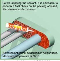
5) A 20 mm thick layer of NOFIRNO® sealant is applied at each side of the conduit. Clean and dry the conduit opening and the pipes thoroughly, and remove any dirt, rust or oil residues before applying the sealant.
