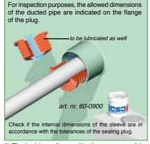
5) The inside surfaces of both segments of the SLIPSIL® sealing plug are then also treated with CSD® lubricant.
