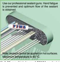
5) A 20 mm thick layer of FIWA® sealant is applied at each side of the conduit. Clean and dry the conduit opening and the cables thoroughly, and remove any dirt, rust or oil residues before applying the sealant.
