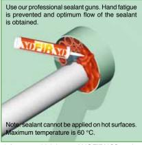
5) A 20 mm thick layer of NOFIRNO® sealant is applied at each side of the conduit. Clean and dry the inside of the conduit sleeve and the outside of the plastic pipe thoroughly, removing any dirt, rust or oil/lubricant residues before applying the sealant.
