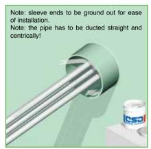
1) Before starting the installation procedure, any dirt, oil residues or welding spots should be removed from the conduit sleeve. For ease of installation, it is advisable to grind out the front side of the sleeve. Ask for the fitting CSD® conduit sleeves.
