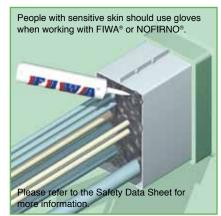
7) Center the RISE® sleeves within the conduit so as to leave 20 mm free space at the front and the back of the transit. A 20 mm layer of FIWA® or NOFIRNO® sealant is applied at both sides of the transit.
