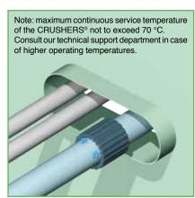
3) Push the RISE®/ULTRA crusher/wrap into the conduit sleeve in such a way as to leave 20 mm free space at the front and back side.
