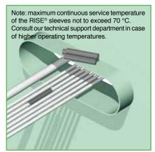
1) The cables can be ducted through the conduit sleeve/frame in random order. It is most important that they are not pulled too tight so as not to hamper their separation when RISE® insert sleeves are inserted.
