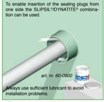
2) Then the inside wall of the conduit sleeve is treated with CSD® lubricant along a distance which approximately corresponds to the length of the SLIPSIL®/DYNATITE® combination.
