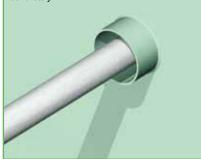
1) Before starting the installation procedure, any dirt, oil residues or welding spots should be removed from the conduit sleeve. For ease of installation, it is advisable to grind out the front side of the sleeve. Ask for the fitting CSD® conduit sleeves.
