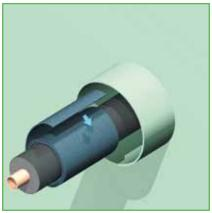
2) A RISE®/ULTRA sheet 210mm wide, 2.5 mm thick is wrapped to the required thickness around the thermal insulation.
