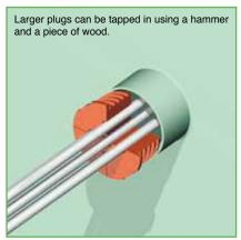
6) The segments of the SLIPSIL® multi- sealing plug are placed around the ducted pipes and then pushed into the conduit sleeve as far as the first serration. The first serration is smaller than the other serrations to make this procedure very easy.
