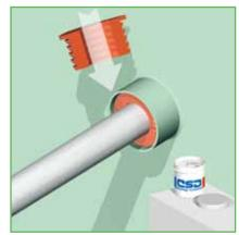
6) The DYNATITE plug should be inserted into the conduit sleeve over a length which corresponds with the length of the second plug. The surfaces of both segments of the SLIPSIL® sealing plug are then treated with CSD® lubricant all around.
