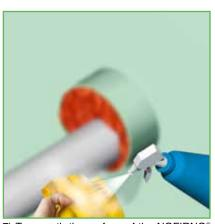
7) To smooth the surface of the NOFIRNO® sealant layer, a cloth is sprayed with water. This prevents the sealant from sticking to the cloth. Note: do not use soap water!
