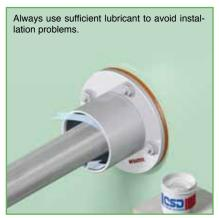
4) The inside wall of the conduit sleeve is treated with CSD® lubricant over its full length. The inlet of the DYNATITE® conduit sleeve is rounded off to avoid any damages to the plug during insertion.
