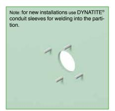
1) When DYNATITE® conduit sleeves for bolting are going to be used, threaded ends have to be welded to the partition in accordance with the hole configuration of the flange of the conduit sleeve.
