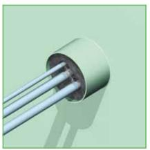
7) Pack the free space inside the penetration with lengths of strip. Compress the filling from time to time firmly to obtain a solid mass of flexible rubber and a good contact with the coaming/sleeve.
