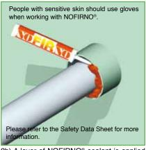
2b) A layer of NOFIRNO® sealant is applied at each side of the conduit. Clean and dry the inside of the conduit sleeve and the outside of the plastic pipe thoroughly, removing any dirt, rust or oil/lubricant residues before applying the sealant.
