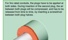
7) The flanged edge of the sealing plug must be flush against the front side of the conduit sleeve. The flange has a distinctive design and is clearly marked with the CSD® and \$(lipsil)® logo.
