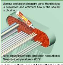
5) A 20 mm thick layer of NOFIRNO® sealant is applied at each side of the conduit. Clean and dry the conduit opening and the cables thoroughly, and remove any dirt, rust or oil residues before applying the sealant.
