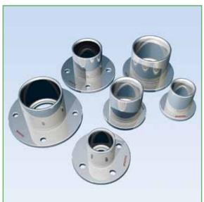
The conduit sleeves are milled to exact internal dimensions from stainless steel 1.4571. The milled sleeves are CDW seam welded to the flanges used for bolting or welding.
