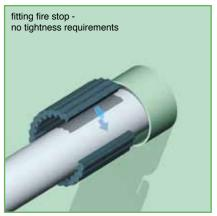
1) The fitting RISE®/ULTRA C-FIT crusher, which is split lengthwise, is folded around the ducted plastic pipe in front of the conduit sleeve
