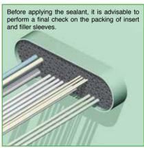
4) Push the insert/filler sleeves into the conduit in such a way as to leave about 20 mm free space at the front. The whole set of insert and filler sleeves should fit tightly into the conduit to provide sufficient mechanical stability.
