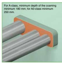
11) For A-class penetrations, the conduit sleeve needs to be insulated only at the insulated side of the bulkhead or at the lower side of the deck. The ducted pipes have to be insulated according to the specifications on the certified drawings.
