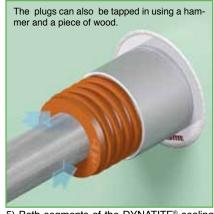
5) Both segments of the DYNATITE® sealing plug are placed around the ducted pipe, then pushed into the conduit sleeve as far as the first serration. Both halves are then pushed by hand evenly, further into the conduit sleeve.
