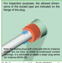
5) Both segments of the DYNATITE® sealing plug are placed around the ducted pipe, then pushed into the conduit sleeve as far as the first serration. Both halves are then pushed by hand evenly, serration by serration, further into the conduit sleeve.
