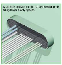
3) The remaining free space in the conduit is filled with RISE® filler sleeves type 27/19 and 18/12. For ease of filling, the RISE® filler sleeves are supplied non-split. The ratio 27/19 to 18/12 should be about 2:1.
