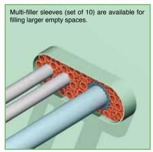
4) The remaining free space in the conduit is filled with NOFIRNO® filler sleeves type 27/19 and 18/12. For ease of filling, the NOFIRNO® filler sleeves are supplied non-split. The ratio 27/19 to 18/12 should be about 2:1. Alternative only filler sleeves type 22/15.
