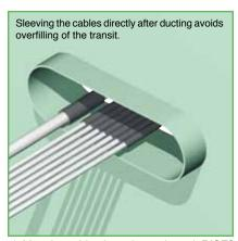
2) After the cables have been ducted, RISE® insert sleeves are applied around each cable. The insert sleeves are split lengthwise and can therefore be placed around the cables in front of the conduit.
