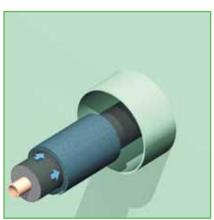
3) Push the crusher wrap into the conduit sleeve in such a way as to leave about 20 mm free space at the front and back side.
