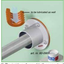
5) The inside surfaces of both segments of the DYNATITE® sealing plug are then treated with CSD® lubricant.
