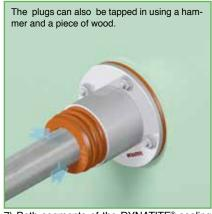
7) Both segments of the DYNATITE® sealing plug are placed around the ducted pipe, then pushed into the conduit sleeve as far as the first serration. Both halves are then pushed by hand evenly, further into the conduit sleeve.
