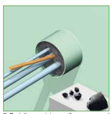
8) Pack the remaining small spaces around the cables with spare pieces of flexible rubber strip. Then press them down firmly with a piece of wood in order to obtain a good contact with the braiding.
