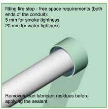
1a) Push the crusher into the conduit sleeve in such a way as to leave about 5 mm, alternatively 20 mm free space, depending on the application, at the front and back side.
