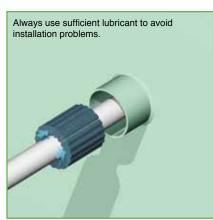
3) In case of a tight fitting crusher, the outside of the crusher and the inner wall of the conduit should be treated with CSD® lubricant for ease of installation. Push the crusher into the conduit sleeve. Check for a tight fit.
