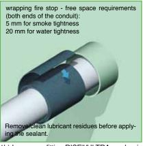
1b) In case no fitting RISE®/ULTRA crusher is available, use can be made of RISE®/ULTRA sheets to be wrapped around the plastic pipe. RISE®/ULTRA wraps are used also for conduit openings which are a bit oversized.
