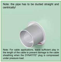
1) Once the DYNATITE® conduit sleeve is welded into the partition, the pipe/cable can be passed through. Before starting the installation procedure, any dirt or oil residues should be removed from the conduit sleeve.
