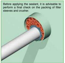
4) Push the NOFIRNO® filler sleeves into the conduit in such a way as to leave about 20 mm free space at the front. The whole set of filler sleeves should fit tightly into the conduit to provide sufficient mechanical stability.
