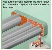
14) When working on larger conduits, the sealant should be applied in two or more parts. Due to the fast curing of the top layer of the sealant, the amount of sealant should not be more than can be finished within 10 minutes.
