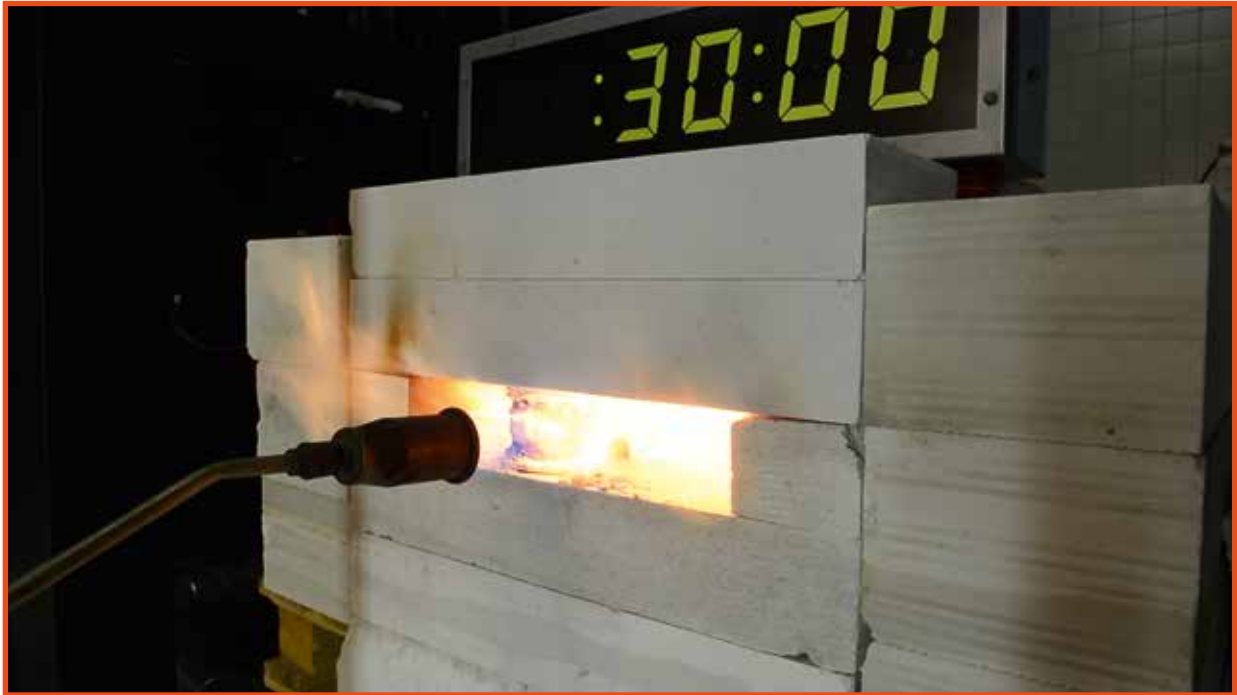
The situation at the end of the test. Temperature on the aluminum pipe 360 °C, far below the melting point of the aluminum.
