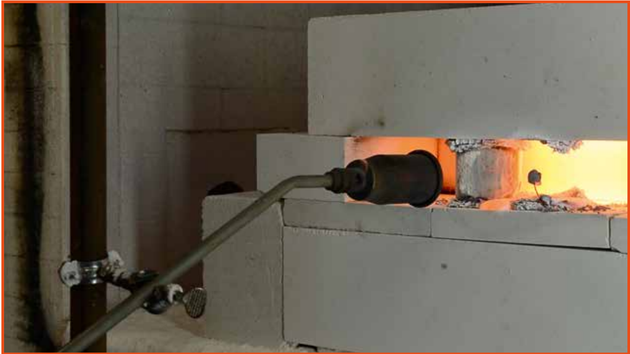
Close-up of the FISSIC® treated test specimen and the char of the NOFIRNO® sealant at the end of the jet test.
