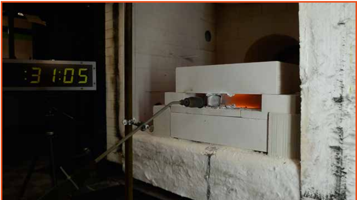
No after-flaming of the FISSIC® coating and NOFIRNO® sealant.
