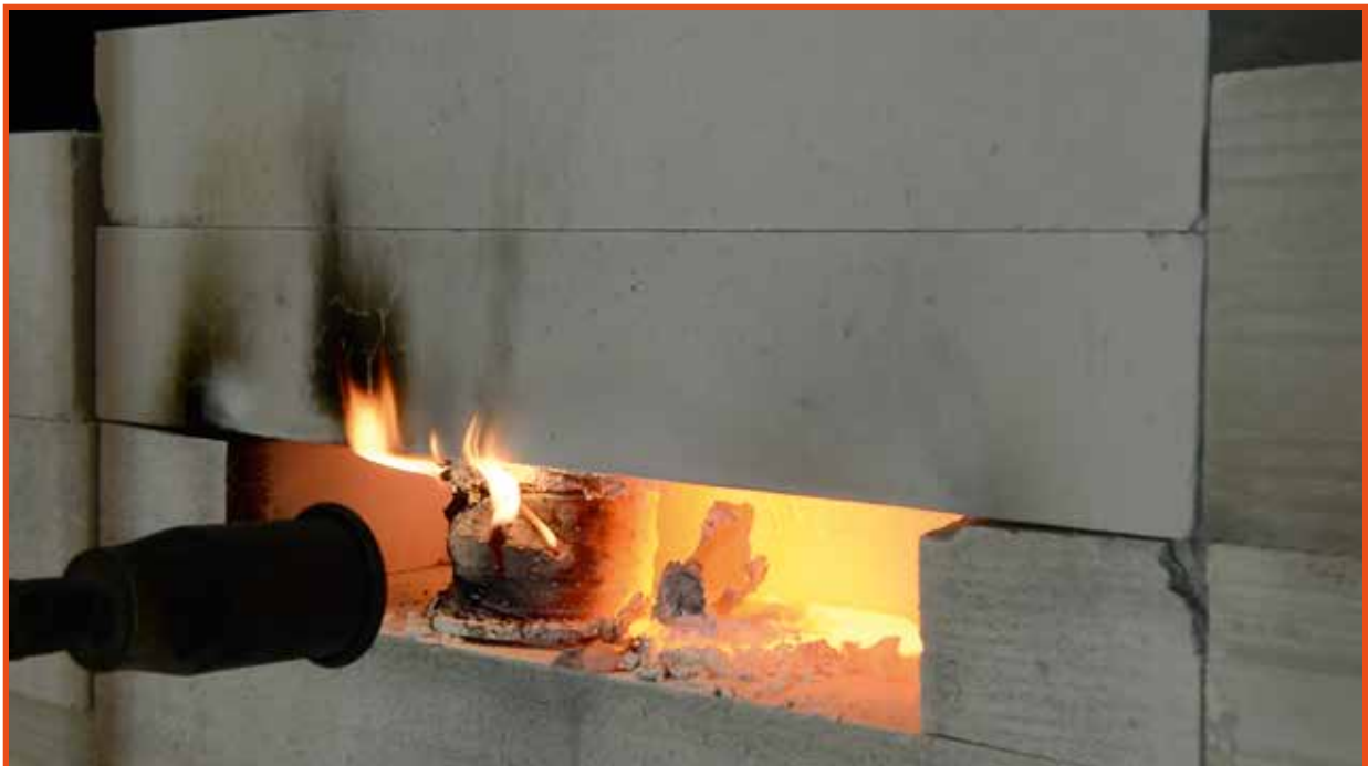
Some after-flaming of the FISSIC® coating is visible after the jet flame has been extinguished. This might have been caused by the fact that the FISSIC® coating probably has not fully cured due to the thickness of the layer.
